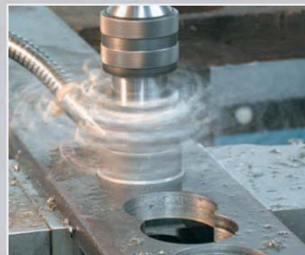
Drilling flat steels
