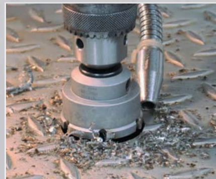
Drilling structured sheet metals
